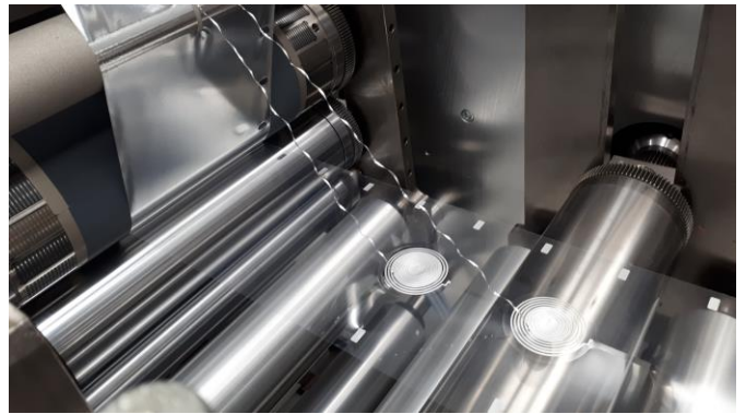
Fig. 2. Die cutting desired shape (top) and removing excess foil (bottom) in a continuous R2R process.
