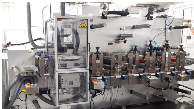
Figure 1. R2R converting line
