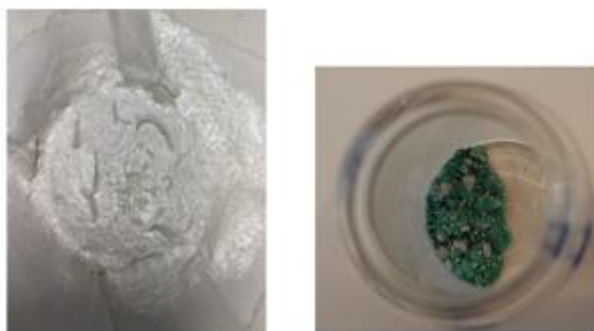
Figure 17. Best experience with printed electronics of two metal layers and one dielectric on one side samples (Left: BHET crystals. Right: separated Ag-ink + dielectric)
