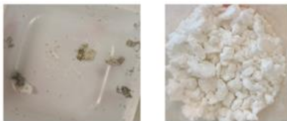
Figure 15. First filter with Ag-ink and unreacted ITENE's sample (left) and BHET crystals (right).
