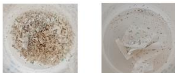
Figure 16. Unreacted PET and Ag-ink using another catalyst in the glycolysis of ITENE samples.
