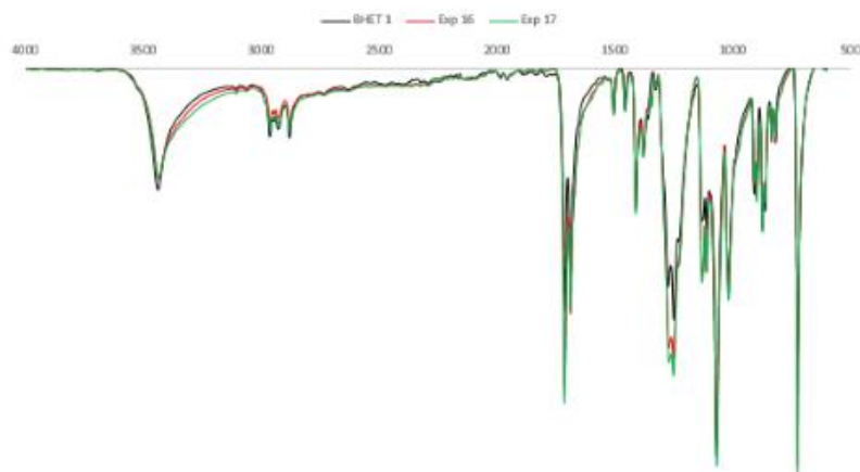
Figure 19. Example of FTIR spectrum of BHET samples (red and green) and reference BHET standard (black)
