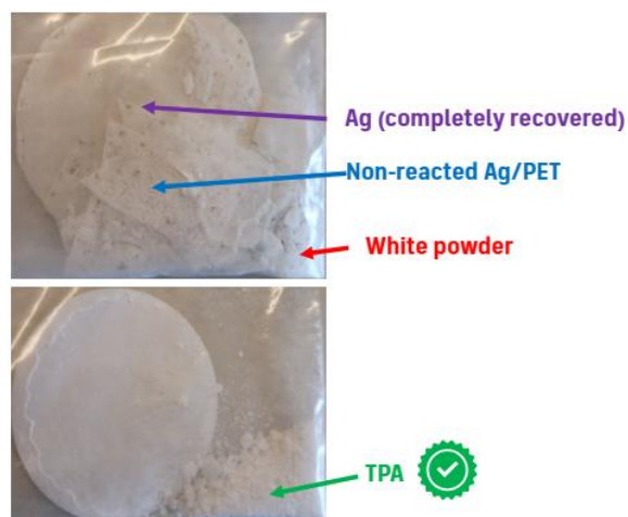
Figure 10. First filter containing Ag recovered, non-reacted Ag/PET and white powder ( \text{Ag}_2\text{SO}_4 ) (above). Second filter containing TPA monomer product (below).
