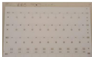
Figure 3. Printed electronic with PET substrate: Ag-based ink sample / White cover layer / transparent PET
