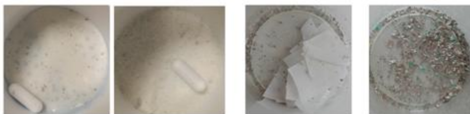
Figure 14. Solid product (two images on the left) and first filter with unreacted PET and Ag-ink (two images on the right) in first glycolysis ITENE samples.
